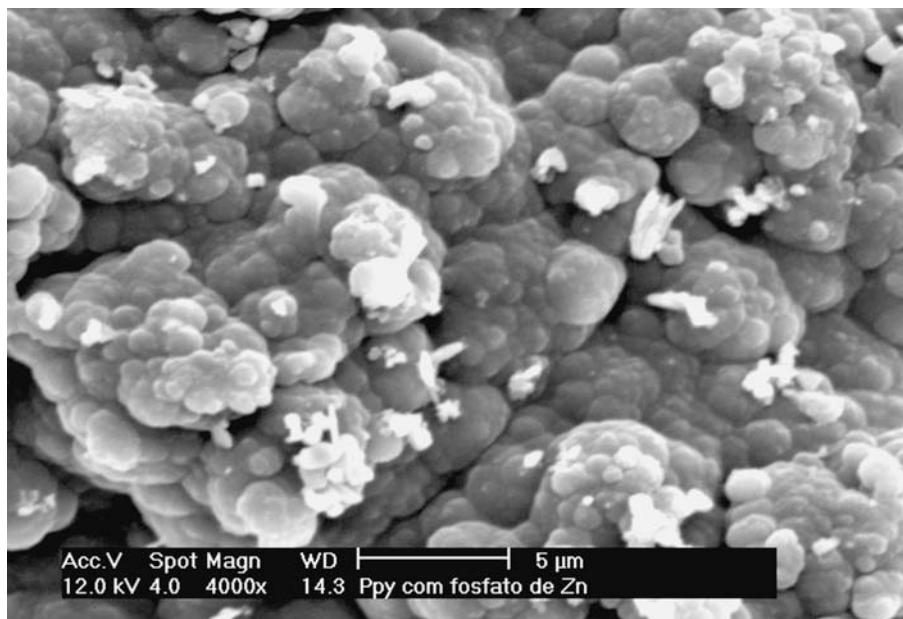
Fig. 7. SEM image of the PPy/zinc phosphate composite film.
